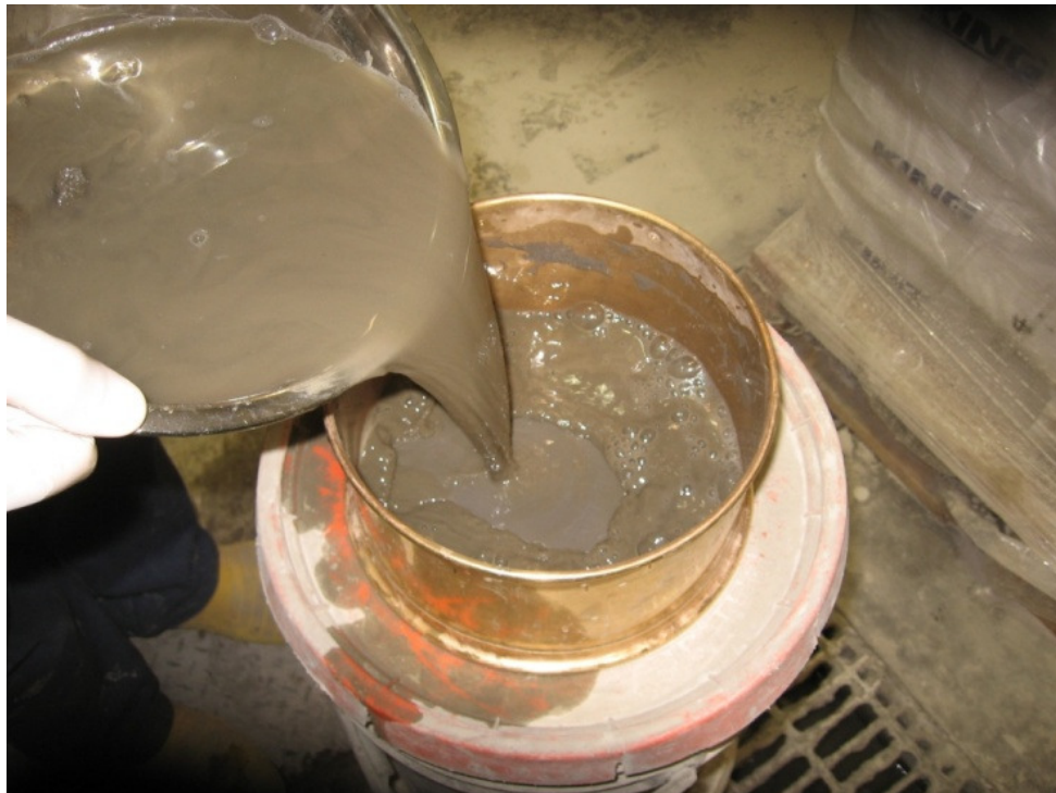
Figure 3.5 : Lavage des granulats (Bolduc 2009)
