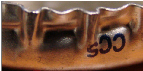
Figure 7.13 Capsule sertie manuellement.
