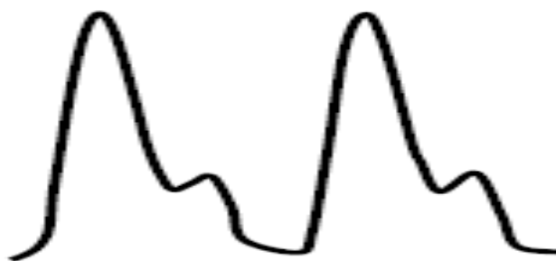
Figure (I.16) La forme de signal PPG [37]
