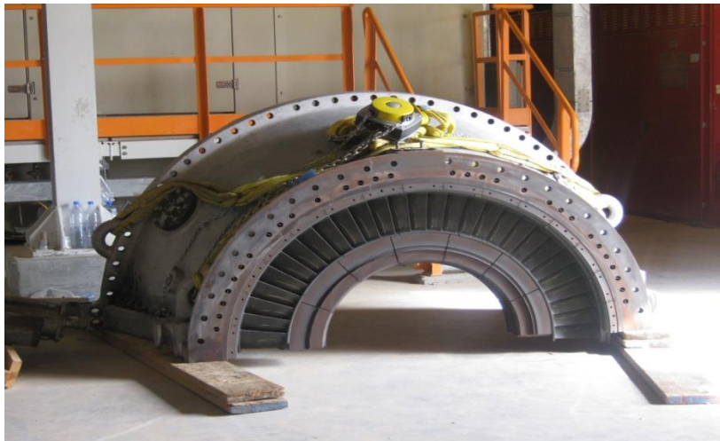
Fig.22 Stator de la turbine
