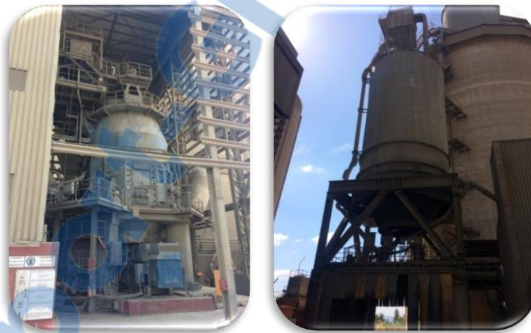
**Figure 9: Broyeur ciment**
