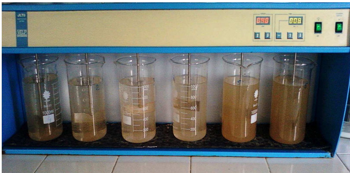
Figure 11: essai de coagulation-floculation
