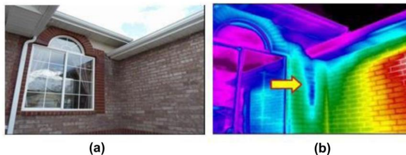
Figure 2. (a) a rgb photo, (b) a ir image that shows moisture penetration near the window.[133]
