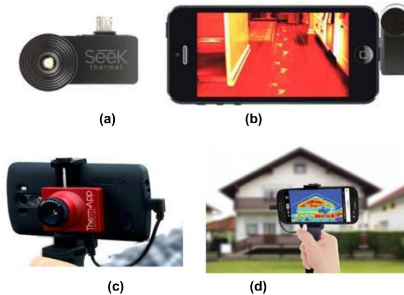
Figure 7. (a) front-view of Seek thermal camera for smartphone, (b) the camera plugged into a smartphone, showing the achieved miniaturisation and the quality of the obtained thermal image,[149] (c) therm-app ir camera for android,[150] (d) a building inspection by therm-app.[151]
