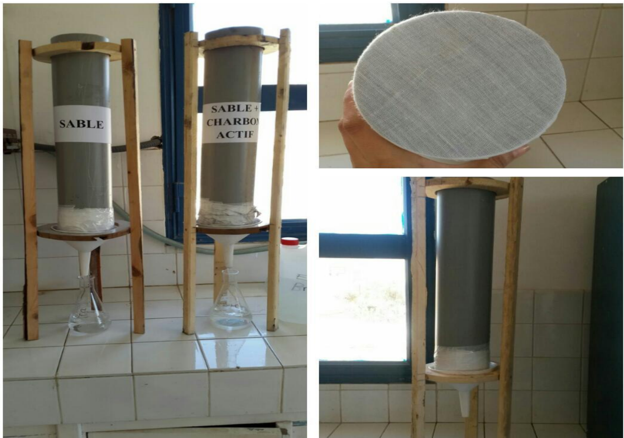
Figure 11: Description des colonnes de filtration
