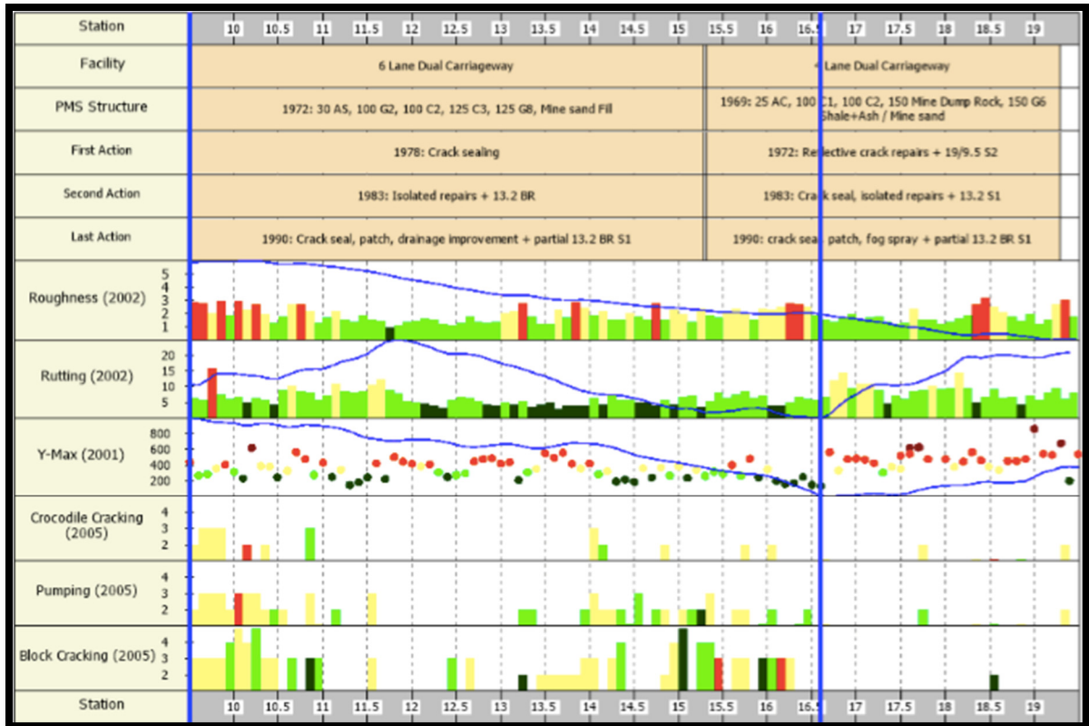
Figure 1.14 Sample itinerary diagram (strip map representation) from South Africa Taken from SANRA (2014)
