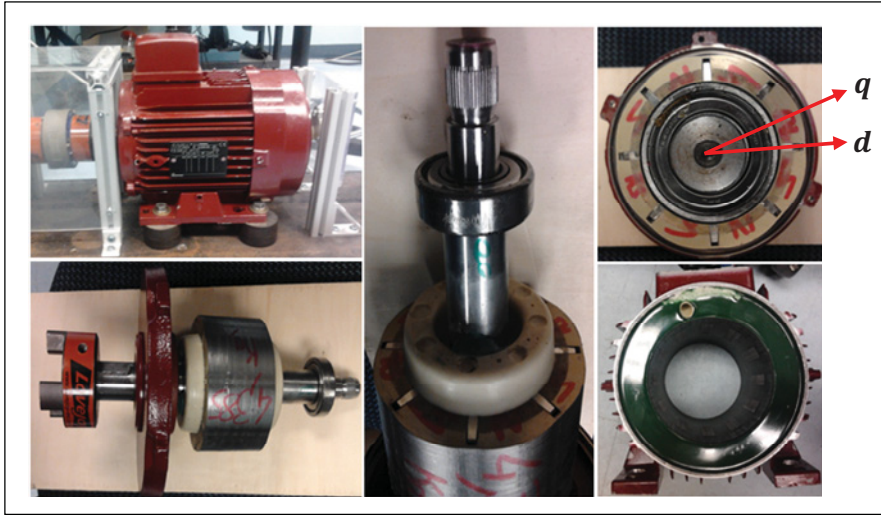
Figure 4.4 Four-pole pairs PMSM used in experiments for testing the HFSI techniques. The permanent magnets are radially inset in the rotor
