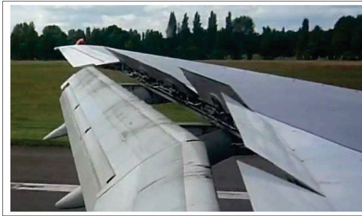
Figure 1.15 Deployed wing flaps on Boeing 757
