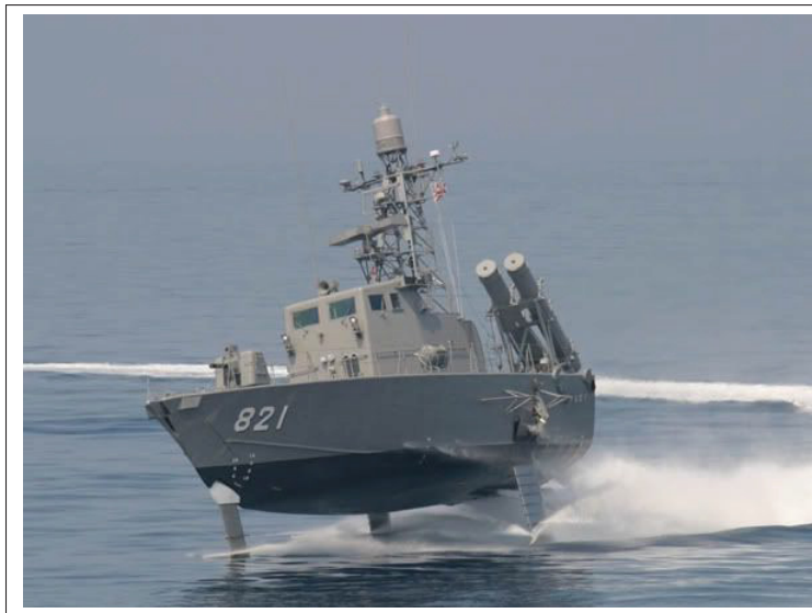
Figure 1.5 Hydrofoiling Spaviero military vessel Image from www.boatdesign.net
