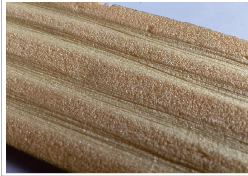
Figure 3.37 Foam Core damage from SMA wires
