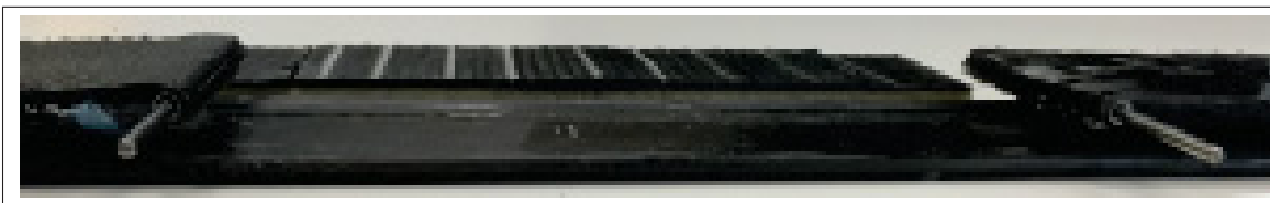
Figure 3.25 Pin Loaded Strap installed on CFRP beam
