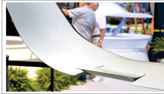
Figure 1.16 FlexFoil technology on wing Image from www.flxsys.com
