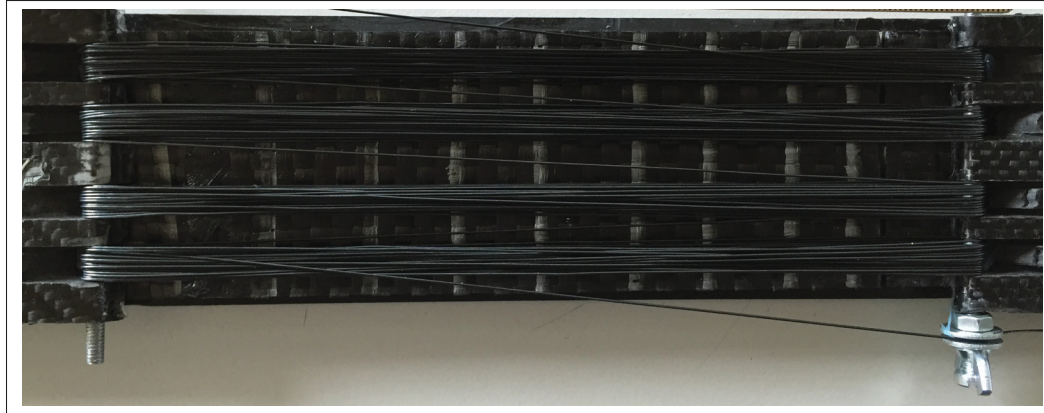
Figure 3.26 SMA wires installed on the PCP
