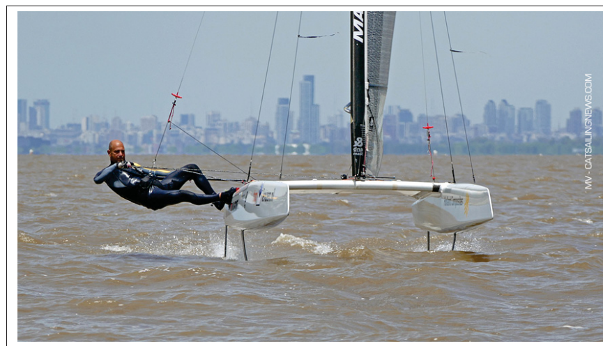
Figure 2.1 Sergio Mehl foiling on DNA AClass with J/Z foils Image from www.catsailingnews.com , using with authorization
