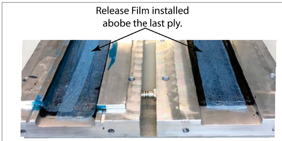
Figure 3.22 Release film installed above the last ply
