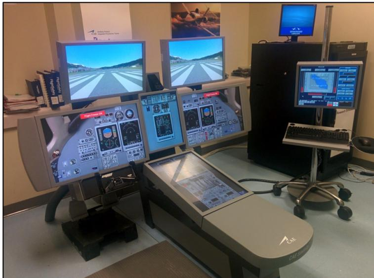
Figure 0-2 Cessna Citation X Research Aircraft Flight Simulator (RAFS)
