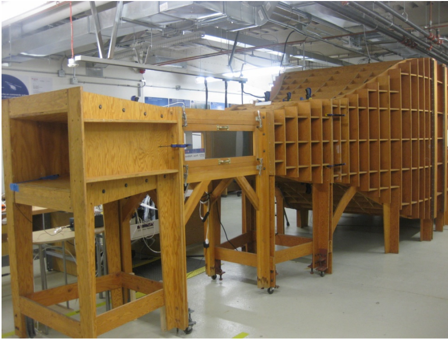
Figure 0.6 Price-Paidoussis subsonic blow down wind tunnel
