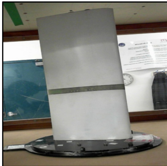
Figure 6.17 ATR-42 morphing wing model
