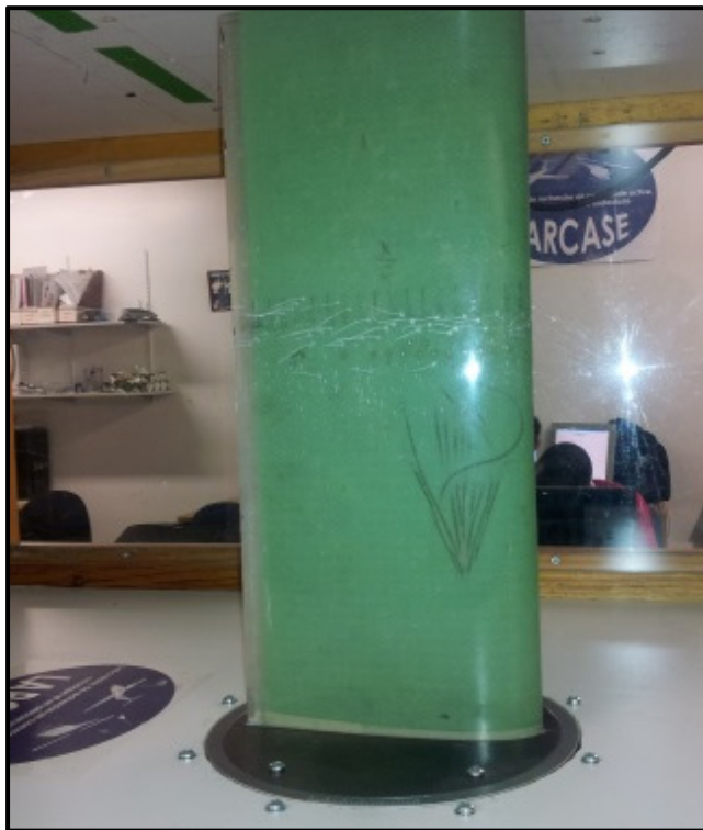
Figure 0.1 Reduced scale of the original wing model of an ATR 42 aircraft
