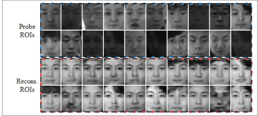
Figure 5.5 A random example of probe ROIs and reconstructed ROIs using the baseline system. The top rows are the probe ROIs and the bottom rows are their corresponding reconstructed face ROIs.
