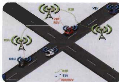
Fig 1 : VANET architecture and communication
