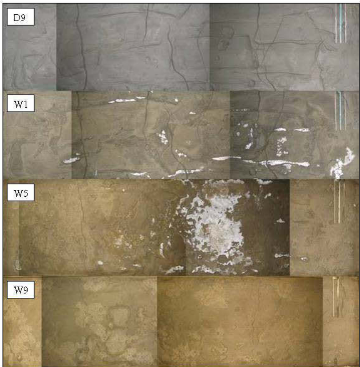
Figure VI.17. Photograph of the surface of the top layer of the model, at the end of the drying period following the deposition of the ninth layer (D9) and at the end of the first (w1), fifth (w5), and ninth (w9), wetting drying/cycles.
