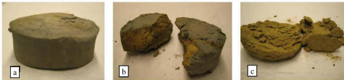
Figure VI.22. Photographs of core samples collected from the physical model: (a) part of a core sample, (b) part of a core sample showing a preferential oxidation pathway, and (c) part of a core sample located near the top of model (oxidized zone). The diameter of a core sample is 5 cm.
