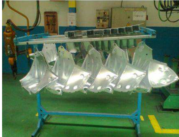
Figure 25 : Solution Poka Yoké d'un support
