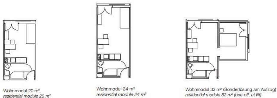
Figure 92 : Plan des appartements_ Modular Apartments [PPA17].
