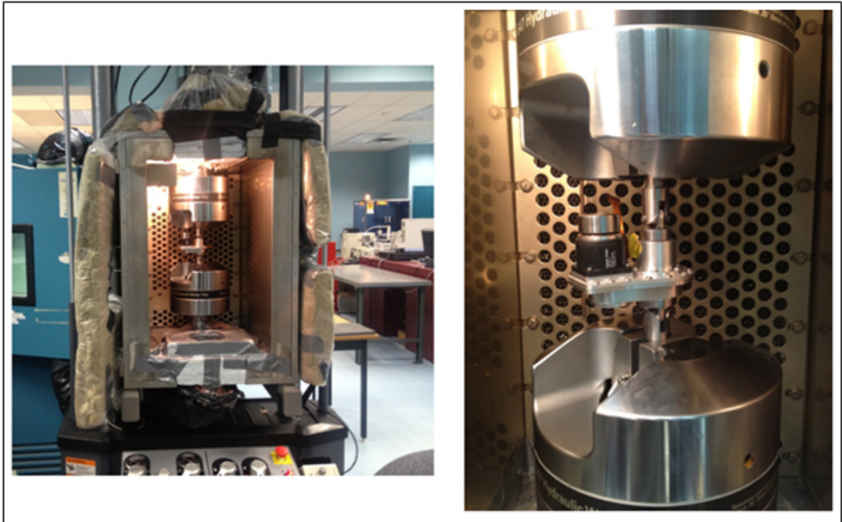
Figure 1.2 Actuator during robustness test at the ETS
