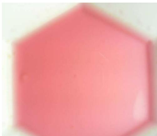
Figure 4.11. Color produced by the reaction of nickel with dimethylglyoxime.
