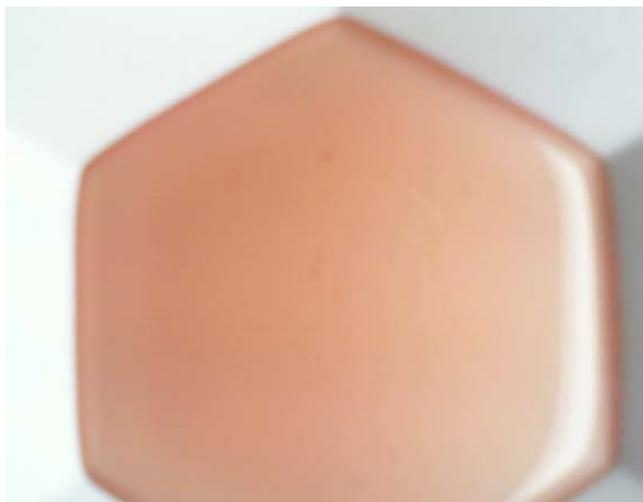
Figure 4.7. Color produced by the reaction of iron with potassium thiocyanate.
