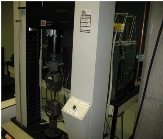
Figure IV.3 Machine de traction LMU-150
