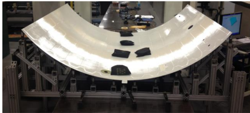
Figure 6-2: An aerospace panel under permissible restrained loads (the weight of black sandbags applied on the surface of part) achieves the functional shape on physical fixture [1].
