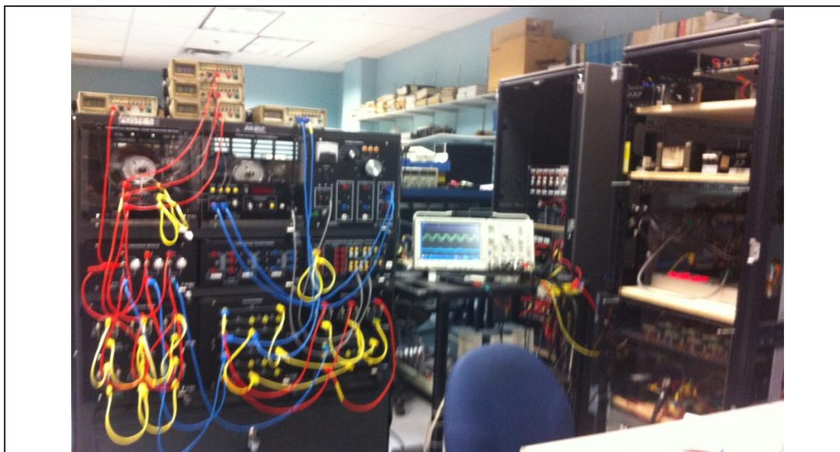
Figure A.1.3 Experimental Setup for hybrid standalone system based on PV array and MHP driven fixed speed SCIG
