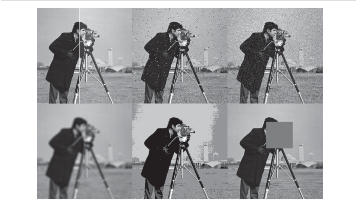
Figure 2.1 MSE vs. perceived quality. This figure shows six different types of degradation applied to the same image. The original is shown in the first frame on the left side of the white line. The degradations from left to right and top to bottom are: DC level shift, salt & pepper noise, Gaussian noise, blur, 4 bits gray-scale resolution and superimposition of a gray square. All cases have nearly identical MSE, but have very different perceived quality.
