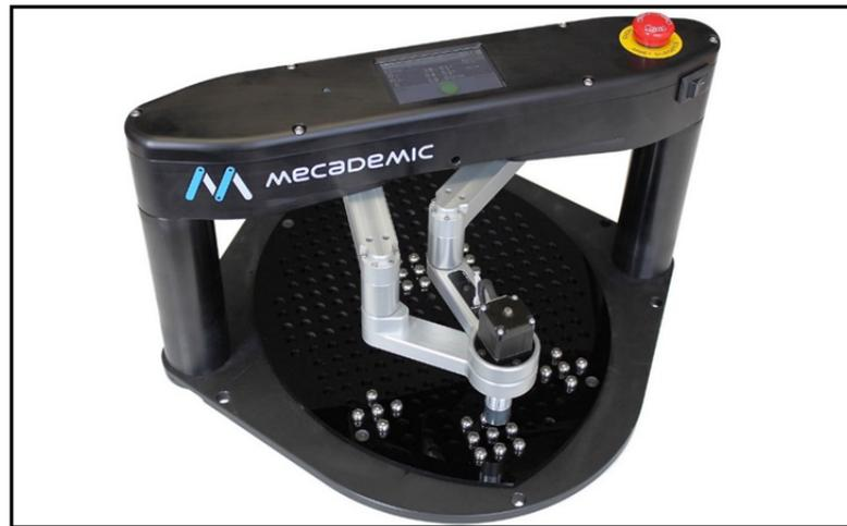
Figure 1.2 DexTar Robot; an example of parallel robot
