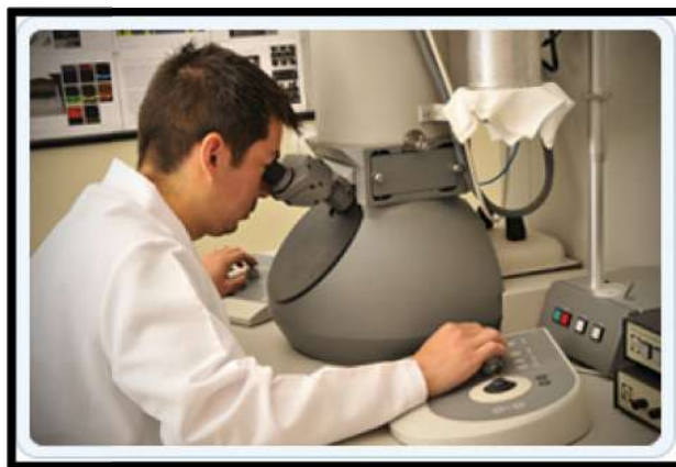
Figure III.4: Appareil de mesures STEM et TEM [64].
