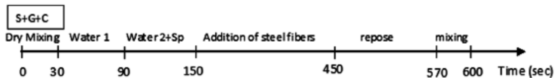
Figure II.2: Mixing procedure for FRSCC
