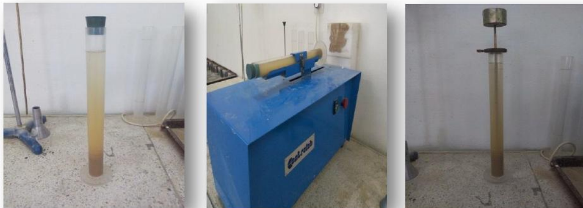
Figure IV.9: Sand equivalent test
