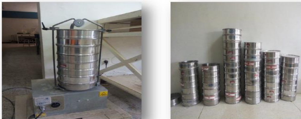
Figure IV.3: Particle size distribution test
