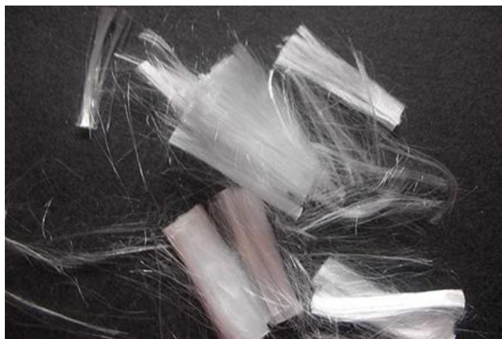
Figure I.7 : Polypropylène fibres (Grueward et al. 2004) [1]
