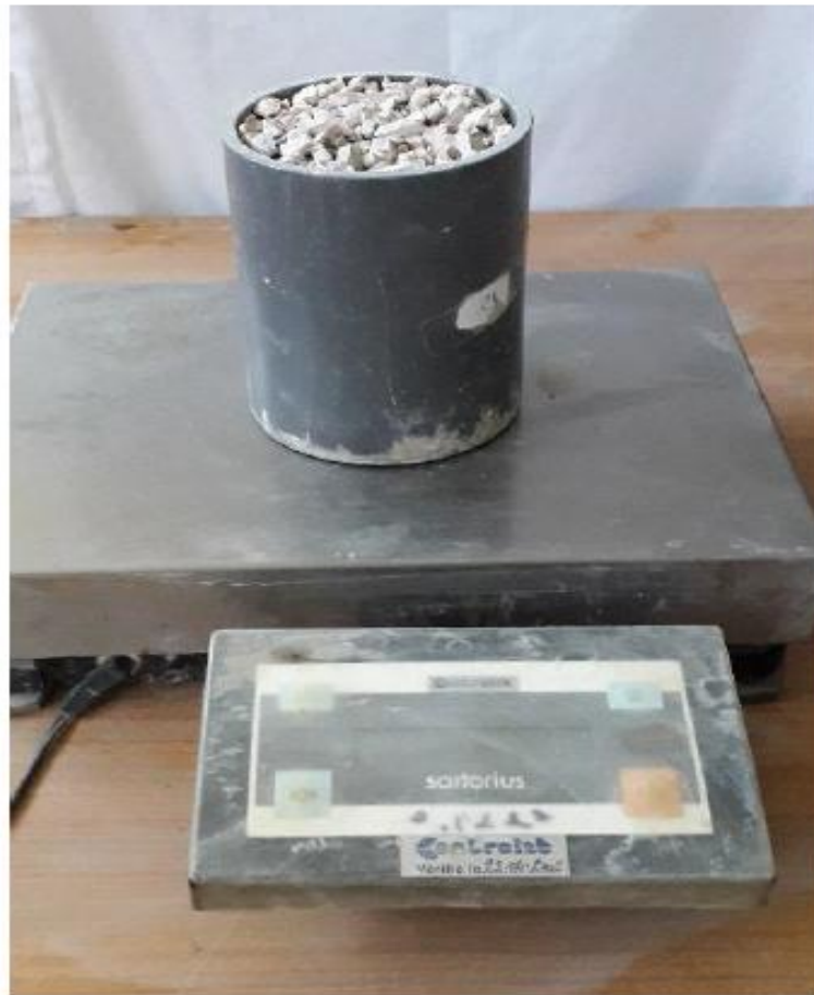
Figure IV.5: Test to measure apparent density
