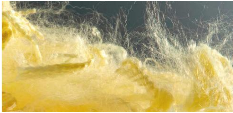
Figure I.6 : Aramid fibres (Grueward et al. 2004) [1]
