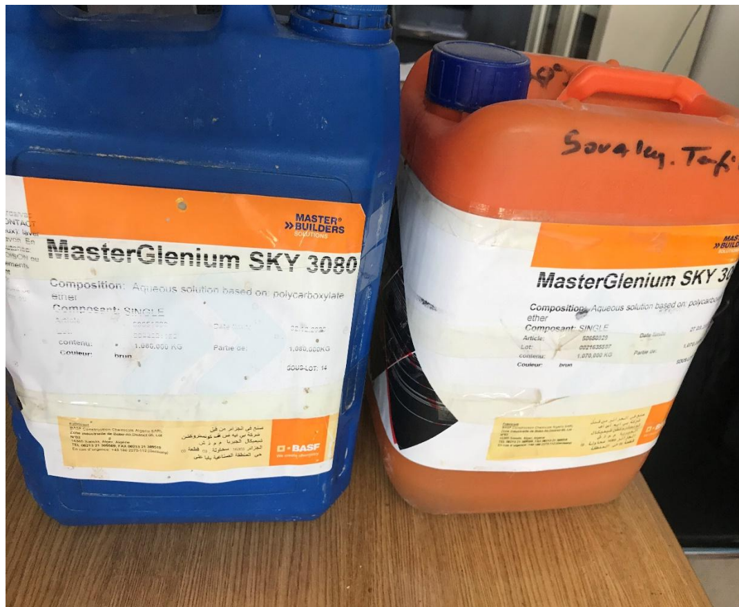
Figure IV.1: Superplasticizer used in the formation of concrete
