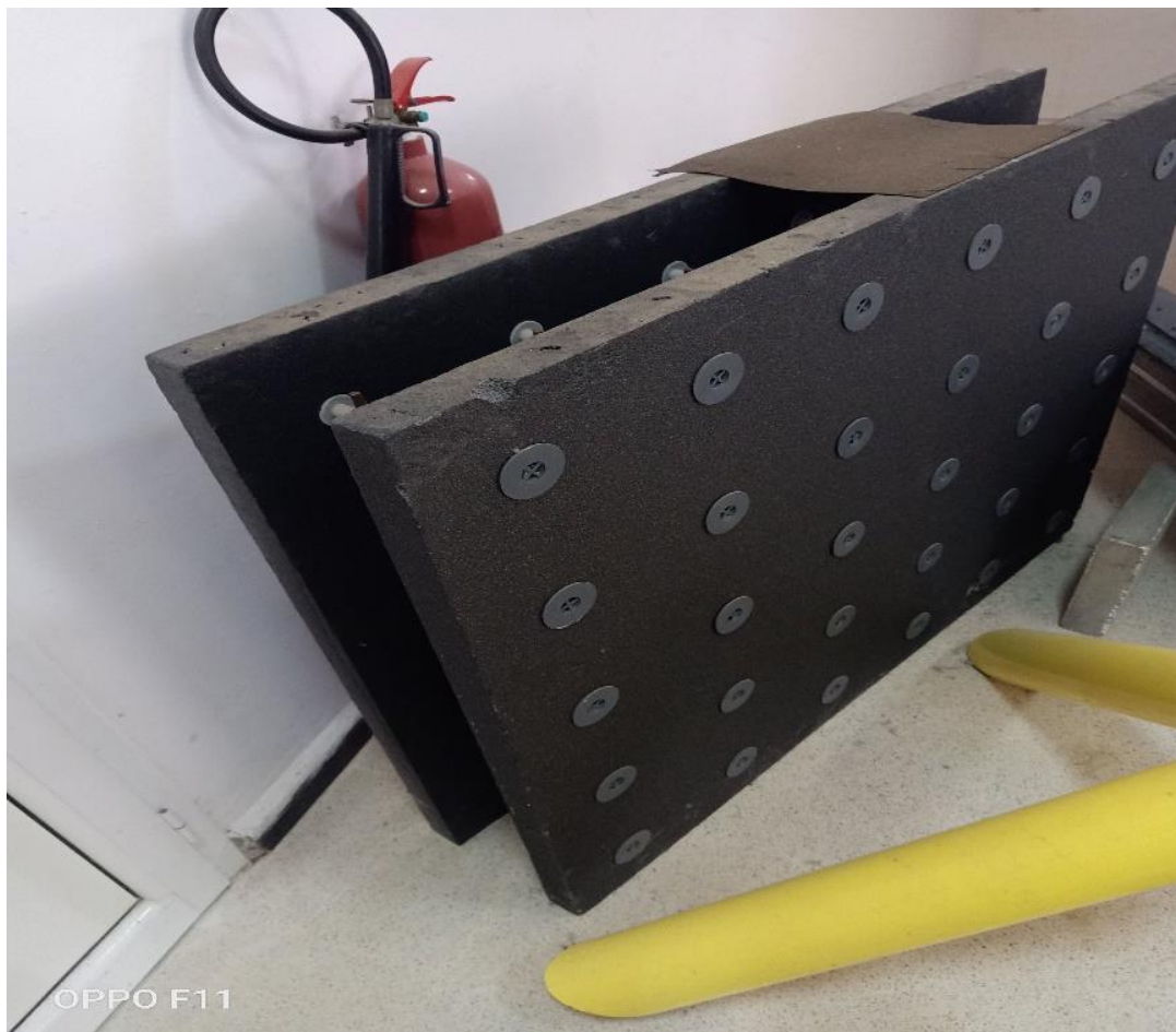
Figure 22 : Extruded polystyrene cnerib /Algiers
