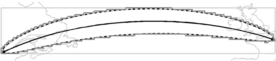
Figure-A I- 12 Comparative illustration, using a geographical projection, of the surfaces corresponding to a routing grid selected using an ellipse for which e = 0.99 and c = 0.25^\circ , and another surface selected using a rectangular window ensuring the same minimal maneuvering surface around the departure and destination airports, for CYUL–LFPG.
