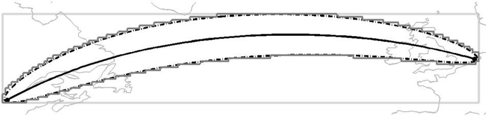
Figure-A I- 11 Comparative illustration, using a geographical projection, of the surfaces corresponding to a routing grid selected using an ellipse for which e = 0.99 and c = 0.25^\circ , and another surface selected using a rectangular window ensuring the same minimal maneuvering surface around the departure and destination airports, for CYUL–EHAM.
