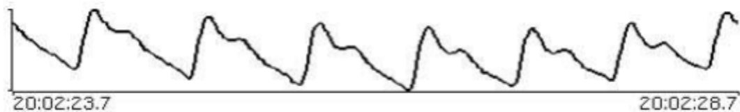
Figure 2.4 Pulsatile Signal while IR or Red light is Transmitted through the Tissue.
