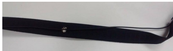
Figure 3.4 Conductive Rubber Cord Fixed on an Elastic Band.
