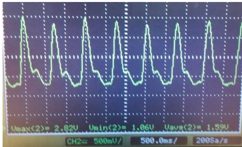
Figure 3.29 Output of the Last Filter as a Response to the IR LED.
