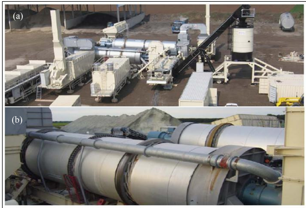
Figure 1.11 Example of the mobile parallel drum plant of AAPPIA Grands Travaux a) overall view & b) closer view of the two parallel drum dryers (the first one for virgin aggregates, the second one for recycled aggregate) Taken from Olard et al. (2008)
