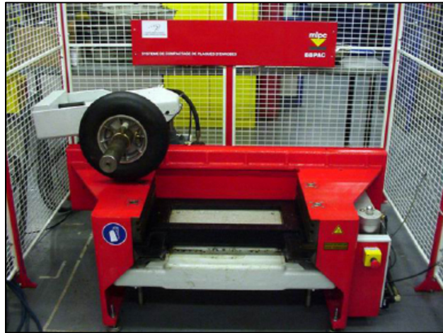
Figure 4.17 Compactor of plates of LCPC
