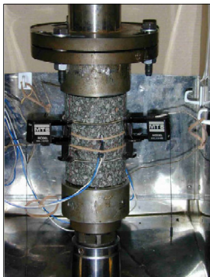
Figure 2.6 Uniaxial tension-compression complex modulus test setup
