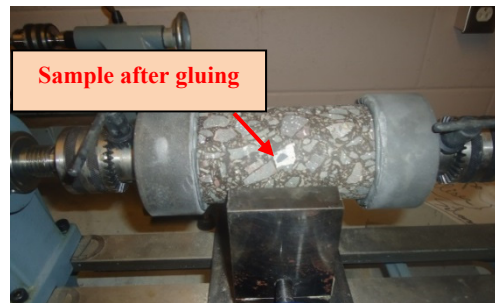
Figure 4.25 Sample after gluing
