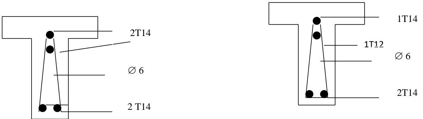
Figure III.2: ferrailage des poutrelles
