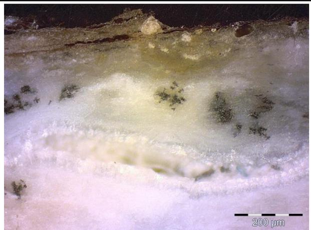
Fig. 9: Micrograph of the metal sample a, from Fig. 2 unetched, dark field, 50x.
