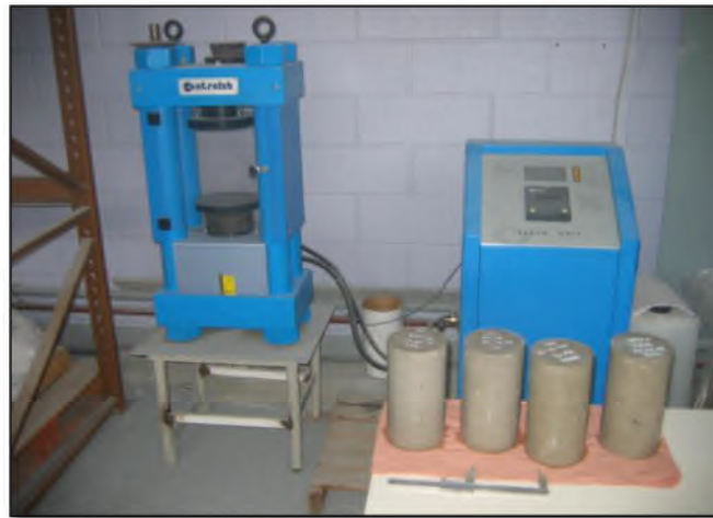
Figure I.2. Essai de compression (Khelifa, 2009).
