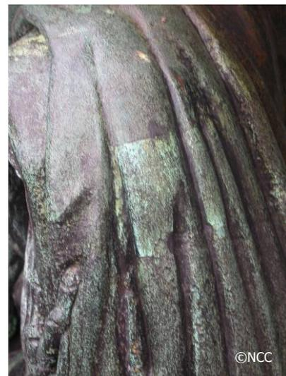
Figure 9 Left: View on a prisoner. One sees clearly the black paint appearing through the green corrosion products.
