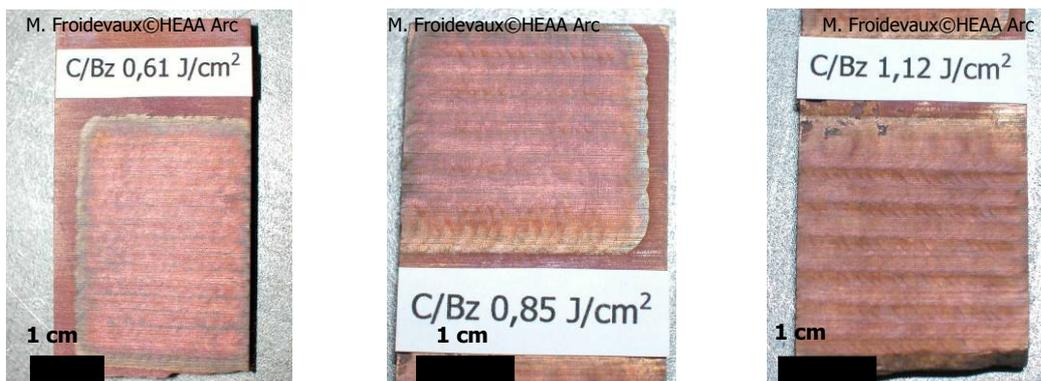
Figure 66 - 67 - 68 Photos of laser cleaned cuprite on bronze at each fluence level 0.61 (left) and 0.85 J/cm<sup>2</sup> (centre) and 1.12 J/cm<sup>2</sup> (right), showing a very low discoloration level to grey.
