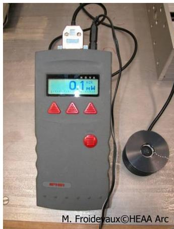
Figure 55 (left) Energymeter and detector.
