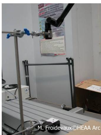
Figure 53 Laser output vertically fixed with clamps for laser cleaning of metal samples (middle) ; handpiece has been removed.
