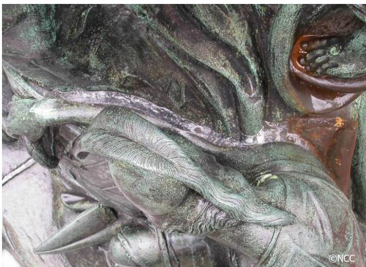
Figure 13 Lead joint clearly visible. Water filling relieves and increasing the corrosion rate.
