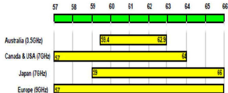
Figure 2-1 Available spectrum in 60GHz band for indoor wireless communication around the world
