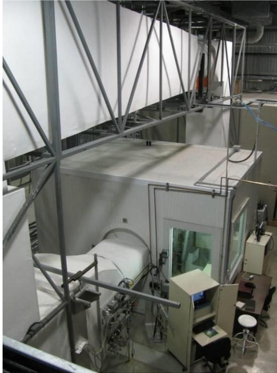
Figure 3-1: CIGELE Atmospheric Icing Research Wind Tunnel
