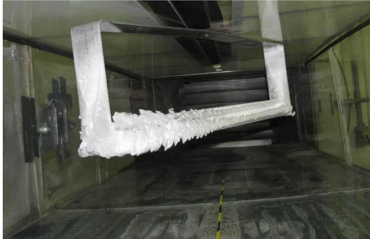
Figure 3-5: Support used for horizontal ice simulation
