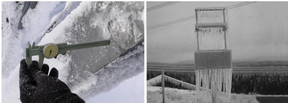
Figure 2-2: Atmospheric ice accretions on transmission line towers
