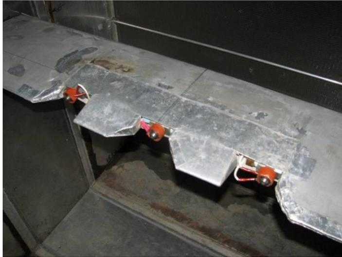
Figure A-2: CAIRWT's Spray Bars with Heating Element
