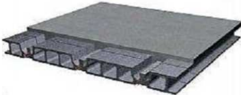
Figure 1.3 Plancher corps creux
