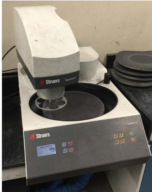
Fig. 3.6 Struers Tegrapol-35 Grinder-Polisher
