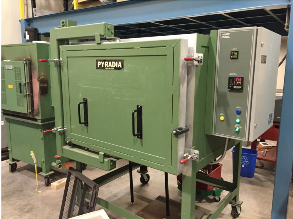
Fig. 3.2 Electrically resistance air-circulating chamber furnace
