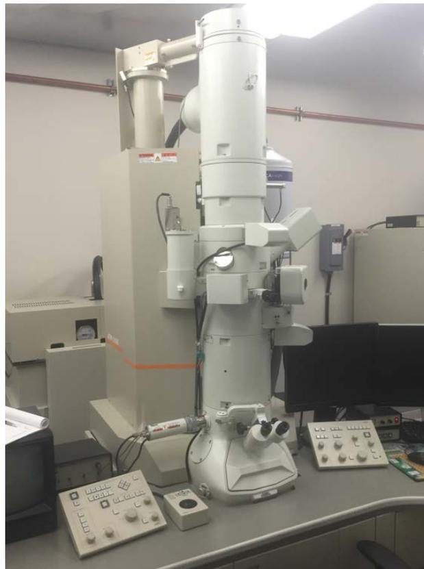
Fig. 3.5 JEM-2100 Transmission Electron Microscope
