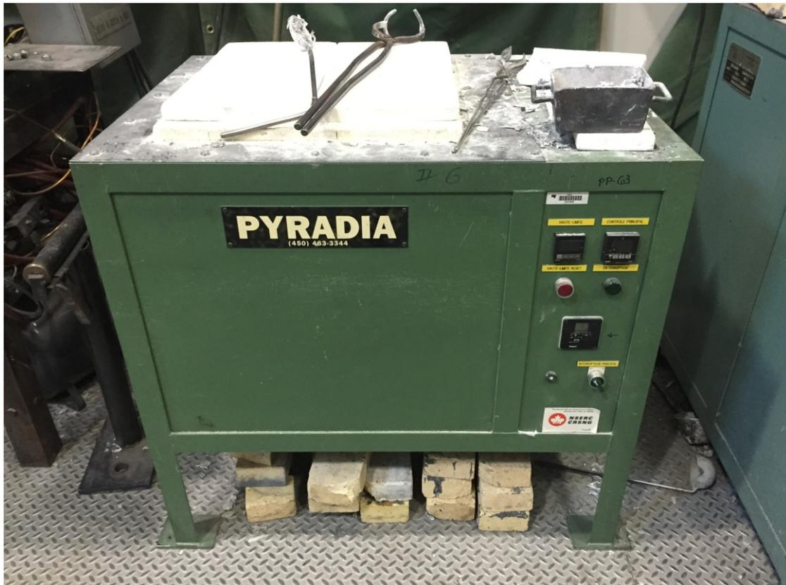
Fig. 3.1 Electrical resistance furnace
