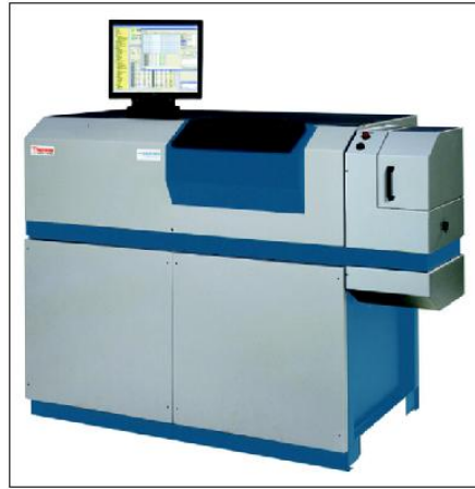
Fig.3.6. ARL 4460 Optical Emission Spectrometer, NRC-ATC laboratories.
