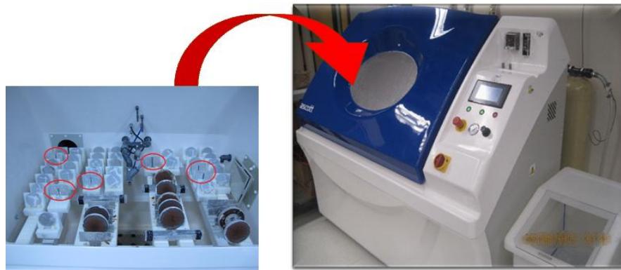
Fig.3.14. A programmable cyclic corrosion test chamber ( Ascott ), NRC-ATC.
