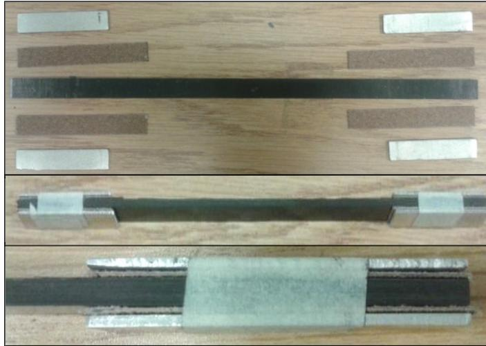
**Figure 2.6: Sample with sandpaper and aluminium tabs**
