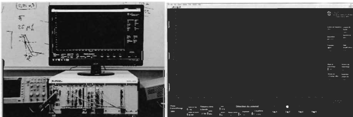
Fig. 5 The reader system implementation using National Instrument PXI-1075 with user interface.
