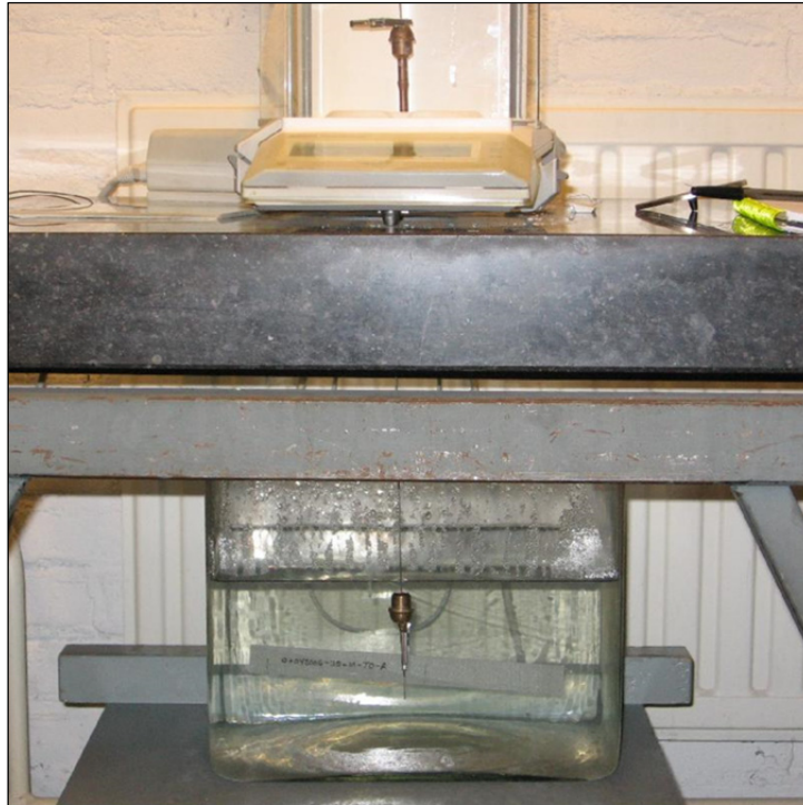
Figure 3.21 Picture of the specific gravity instrumentation
