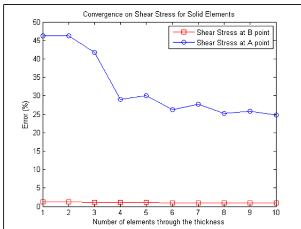
Figure 5.8 Convergence on shear stress for solid elements
