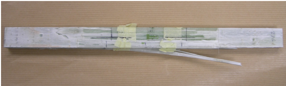
Figure 3.43 Example of the failure for thicker UD specimens under longitudinal tensile load using lateral supports
