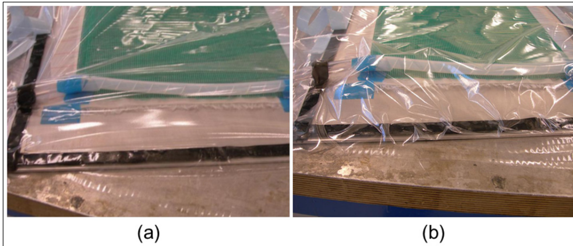
Figure 3.7 Vacuum bag over a thin laminate setup: (a) Free of ribs and (b) With ribs
