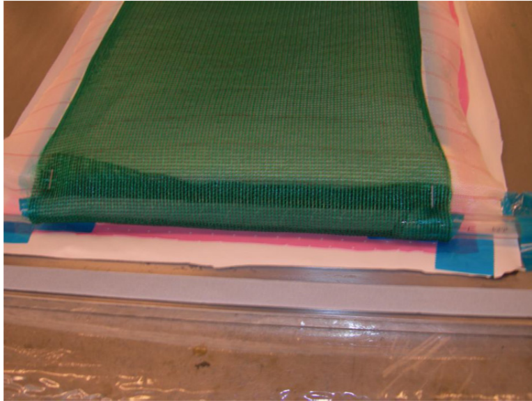
Figure 3.11 Inlet tube installation for a thick laminate
