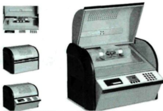
Figure 1.4. Liquid dielectric test set.
