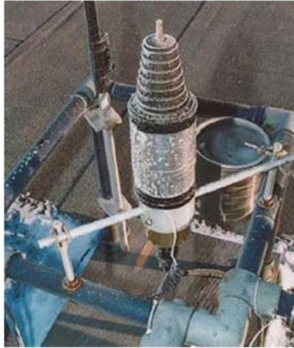
Figure 1.1. A Hydro-Quebec icing-rate meter (AMIL-UQAC).
