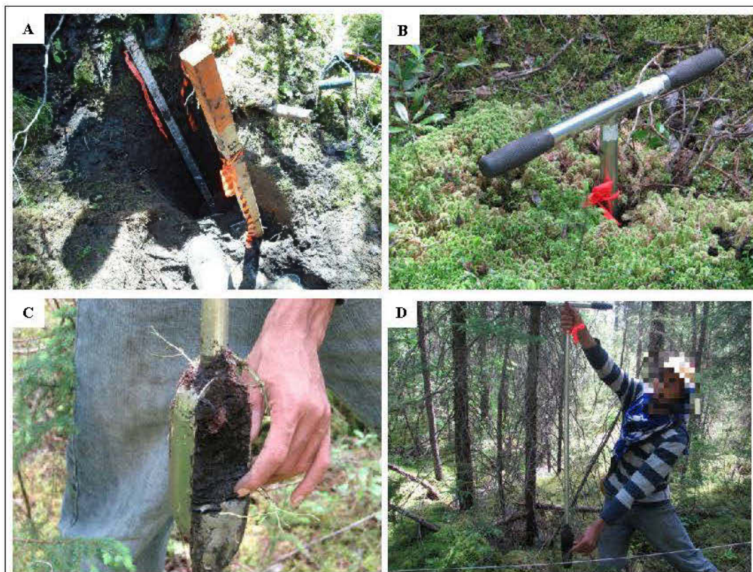
Figure 5.3. Photographs of organic layer measurements within each sample plot made by manual probing. In each plot, a soil pit was dug (centre; A) and an anger was bored through the organic layer until the mineral soil was encountered (four cardinal directions; B); then clearly identified (pointer finger on C); and measured as the distance between the organic layer surface and the mineral soil interface (distance between marker flag and index finger on D).
