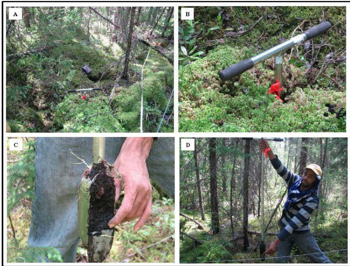
Figure 2.2. Photographs from the study area. At each sampling point, the auger was bored through the organic layer until the mineral soil was encountered (A and B) and then the depth to mineral soil (represents the OLT) was clearly identified (pointer finger on C) and measured (distance between flag mark and pointer finger on D).
