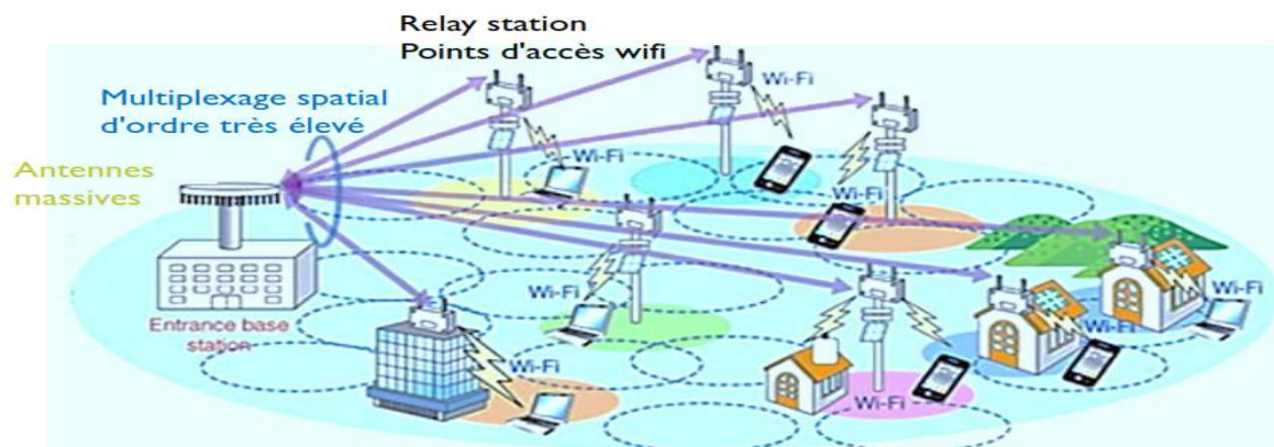
Figure 19 : La technologie MIMO massive [B3]
