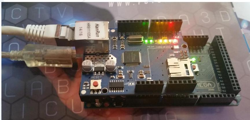
Figure 9- ArduinoMéga 2560c + Ethernet shield [N4]
