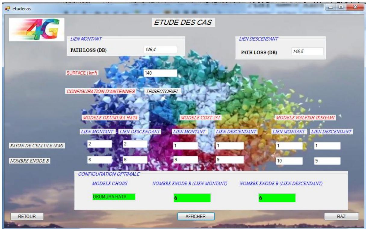
Figure 62: Interface ETUDE DE CAS Configuration optimale
