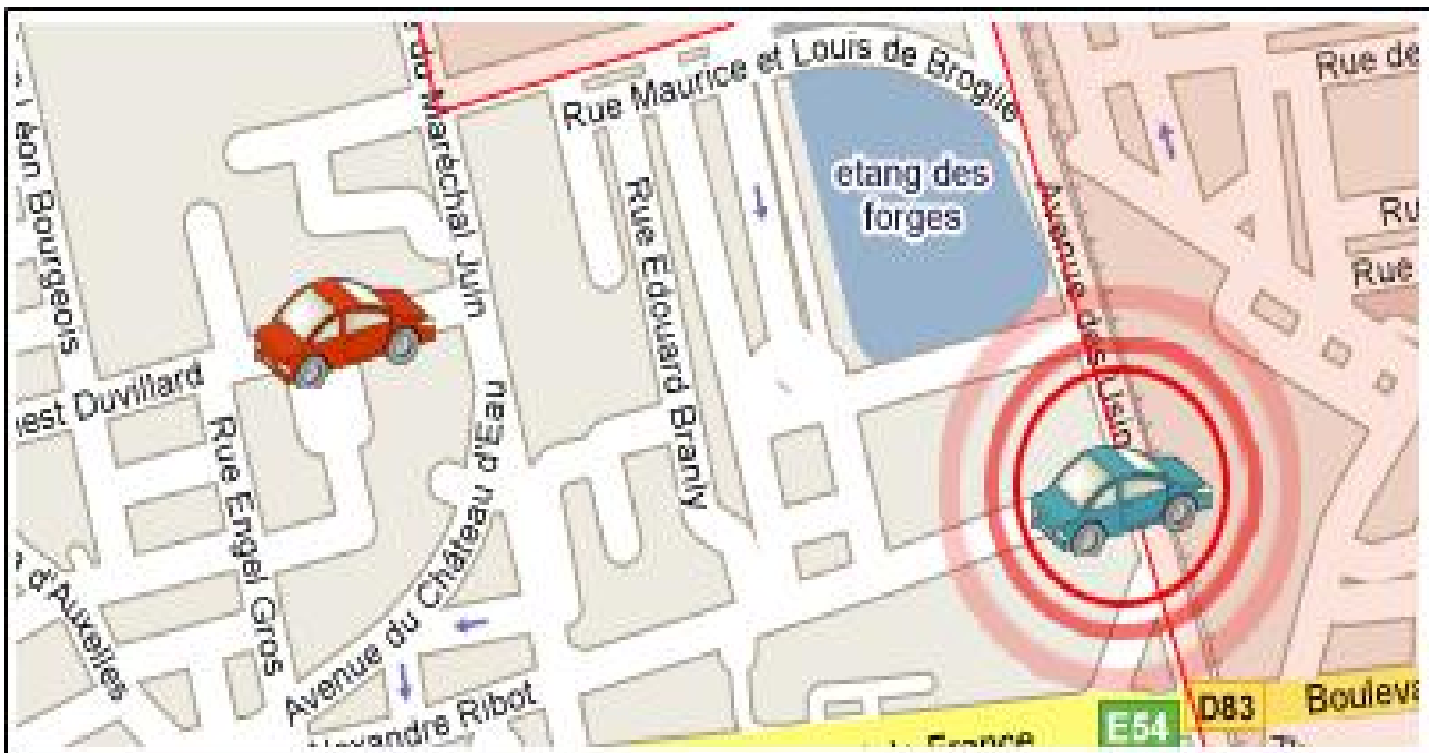
Figure 3-2: Exemple de Geofencing
